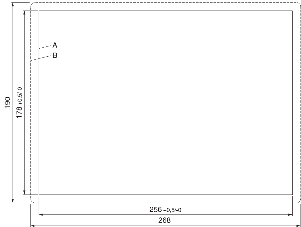
Figure 2-4 Mounting cutout (dimensions in mm)
