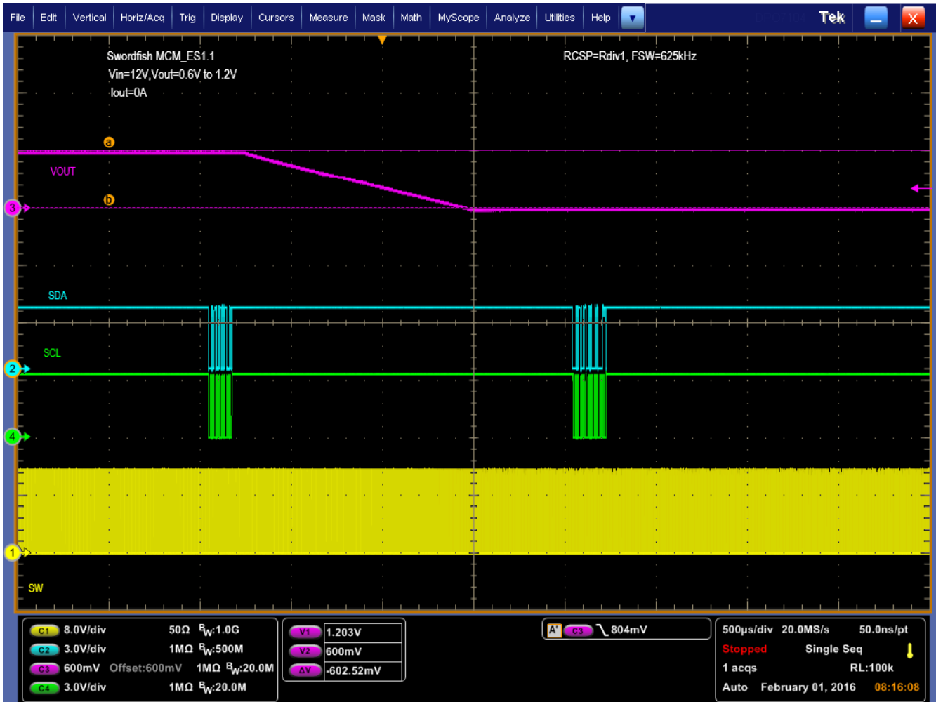
Figure 11-5. PMBus V_{OUT} Step-Down = 1.2 V to 0.6 V at 0 A
