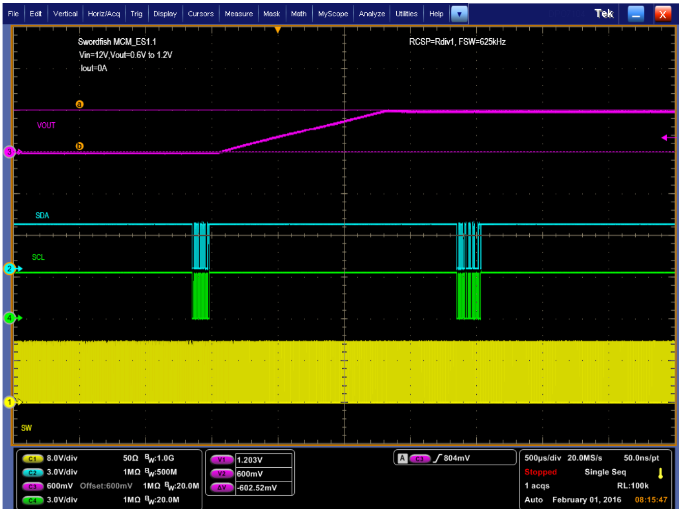
Figure 11-4. PMBus V OUT Step-Up = 0.6 V to 1.2 V at 0 A
