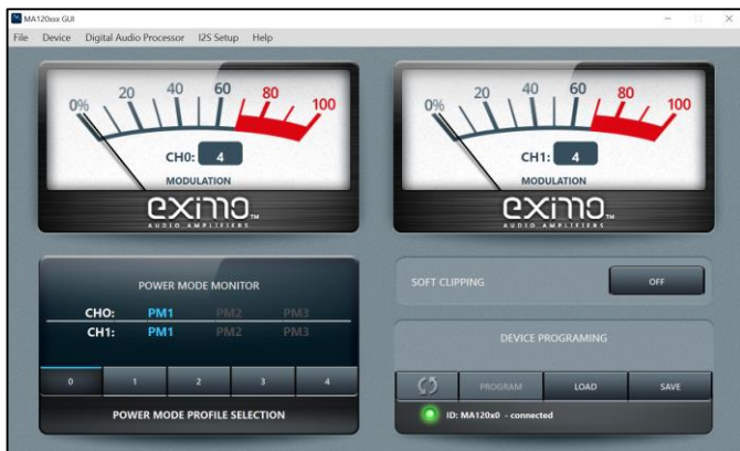
Figure 9. MA120xx control software interface
