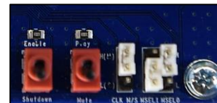
Figure 6. Toggle buttons set to “mute” and “shutdown”
