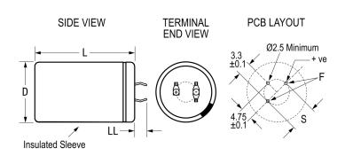
**General Information** Series ALC80 Dielectric Aluminum Electrolytic Description Snap-In, Aluminum Electrolytic RoHS Lead 3 Pin Short AEC-Q200 No Halogen Free Yes Component Weight 80 g Notes Dimensions D And L Include Sleeving. Shelf Life 156 Weeks
