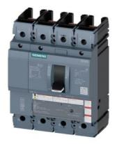
circuit breaker 3VA5 UL frame 250 breaking capacity class M 35kA @ 480V 4-pole, line protection TM210, FTFM, In=90A overload protection Ir=90A fixed short-circuit protection Ii=10 x In N conductor protection 100% without connection
