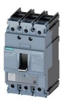
circuit breaker 3VA5 UL frame 125 3-pole, starter protection TM120M, AM, In=50A without overload protection short-circuit protection Ii=3...7 x In cable connection on both sides
