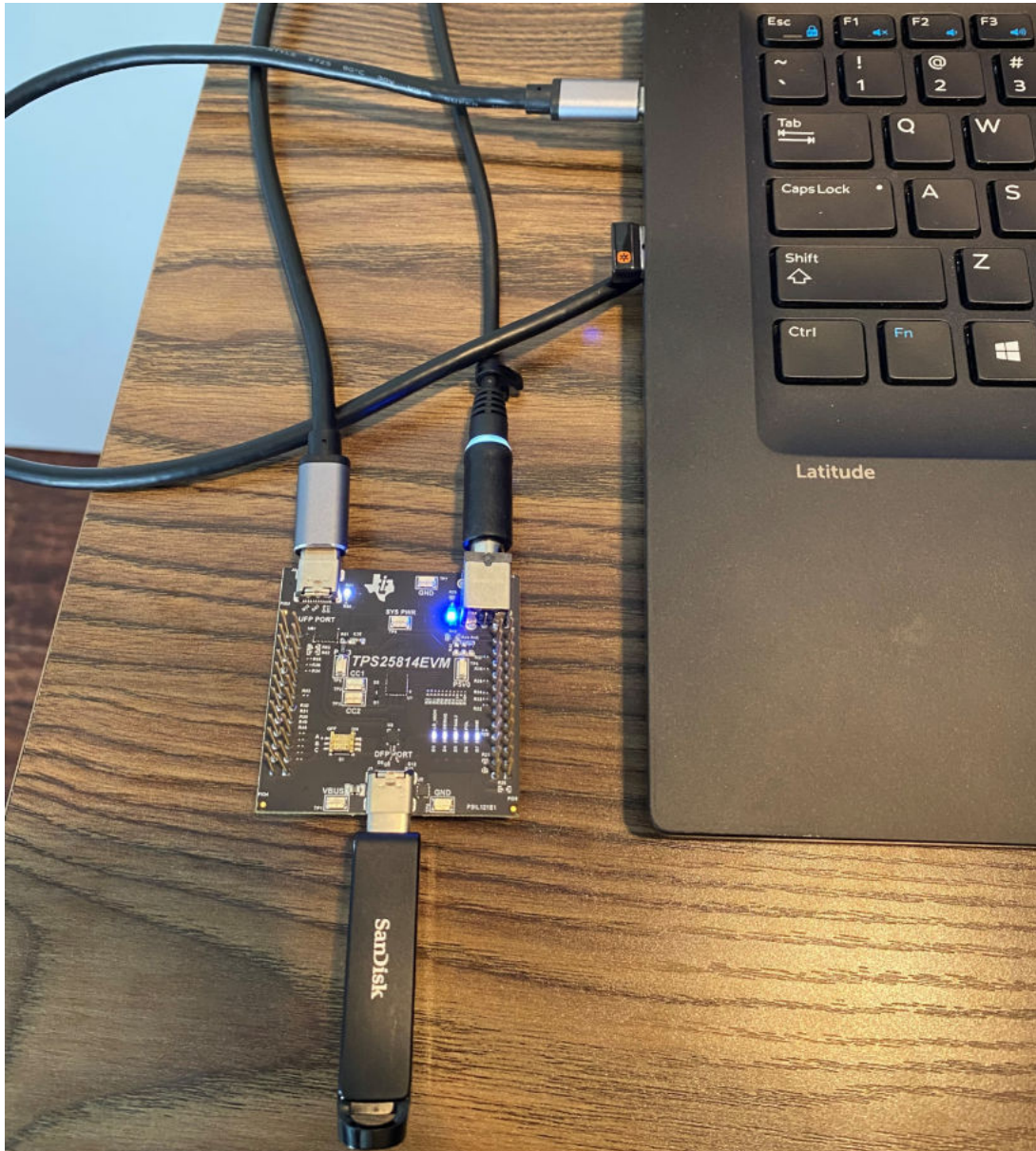
Figure 4-1. USB3 Testing on TPS25814EVM
