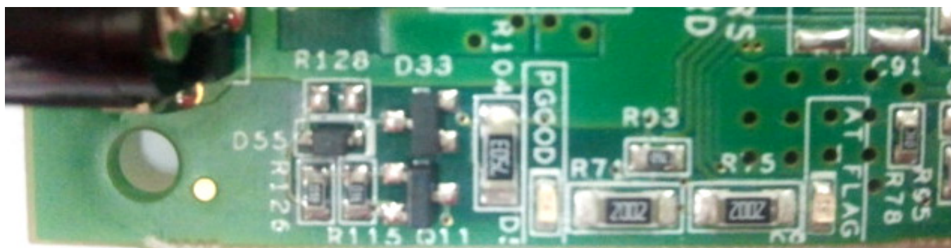
Figure 5: Power_Good LED Indication D5
