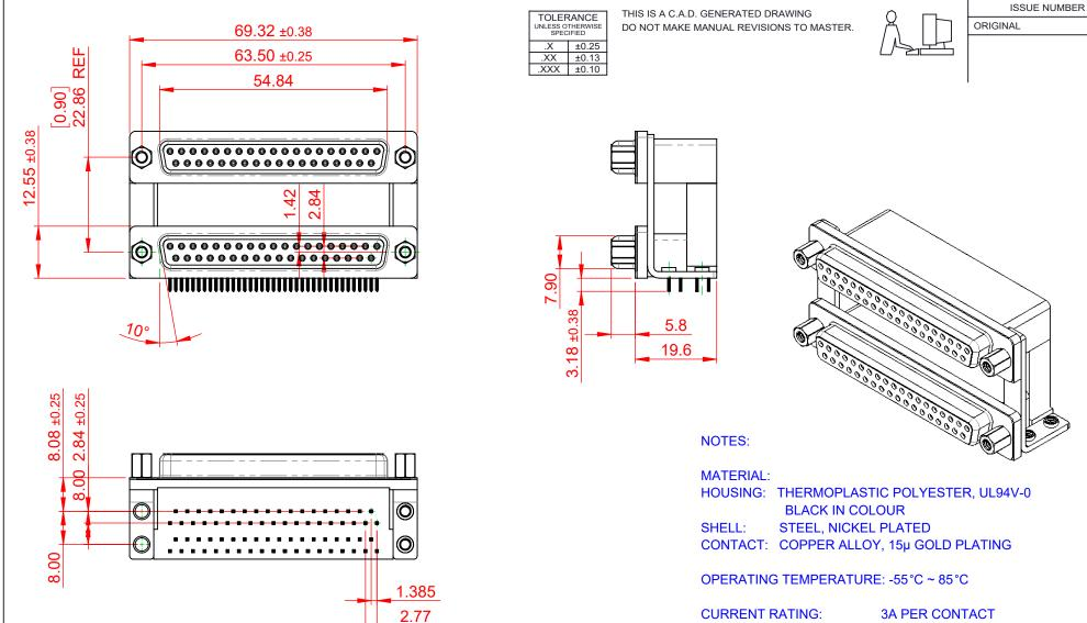
**CURRENT RATING: 3A PER CONTACT** 25mΩ MAX. CONTACT RESISTANCE: INSULATOR RESISTANCE: 5000MΩ min. DIELECTRIC WITHSTANDING VOLTAGE: 1000V AC rms
