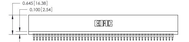
745 Series Ultra-Mate Card Edge Connector - Press Fit Part Number: 745-047-520-101
