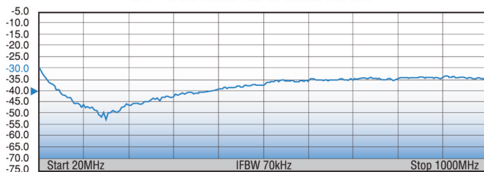
S11 TYPICAL RETURN LOSS (dB)
