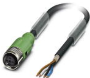
Sensor/actuator cable, 4-position, Variable cable type, shielded, free cable end, on Socket straight M12 SPEEDCON, A-coded, cable length: Free input (0.2 ... 40.0 m)
