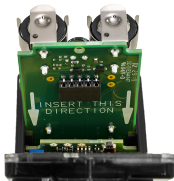
Figure 1: Q45 battery board
