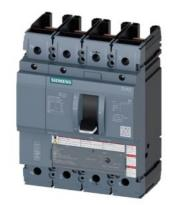
circuit breaker 3VA5 UL frame 250 breaking capacity class H 65kA @ 480V 4-pole, line protection TM230, FTAM, In=250A overload protection Ir=250A fixed short-circuit protection Ii=5...10 x In N conductor protection 100% without connection
