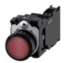
Illuminated pushbutton, 22 mm, round, plastic, red, pushbutton, flat, momentary contact type, with holder, 1 NO+1 NC, LED module with integrated LED 24 V AC/DC, spring-type terminal, Z=20-unit packaging
