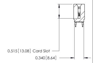
ACAD REFERENCE NO. 746 Series Ultra-Mate Card Edge Connector - Press Fit DRAWN: J.LEE Part Number: 746-054-560-201 CHECKED: **EDAC INC** SCALE: THESE DRAWINGS AND SPECIFICATIONS ARE THE PROPERTY OF EDAC INC.,AND TORONTO, ONTARIO SHALL NOT BE REPRODUCED, OR COPIED DRAWING NUMBER CANADA OR USED AS THE BASIS FOR THE 746-ENG MASTER MANUFACTURE OR SALE OF APPARATUS YOUR CONNECTION TO QUALITY & SERVICE WITHOUT WRITTEN PERMISSION.
