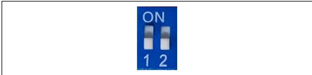
FIGURE 3-1: SW9 IN FLASH APPLICATION MODE
