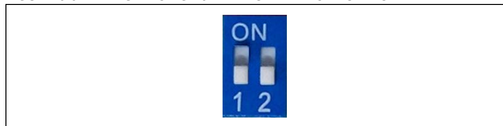
FIGURE 3-37: SWITCH SW9 IN FLASH APPLICATION MODE
