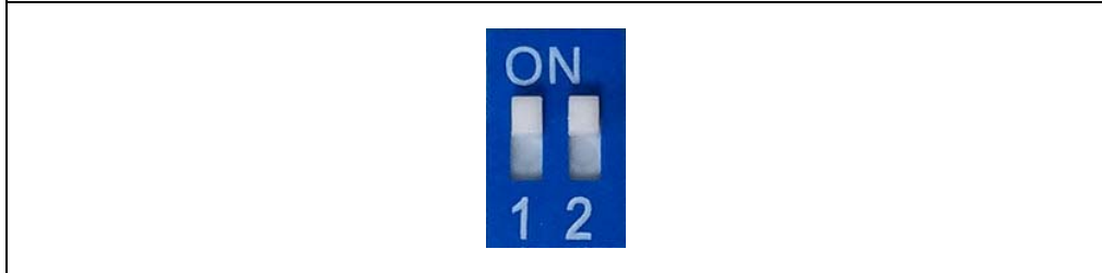
FIGURE 3-38: SWITCH SW9 IN ROM TEST MODE
