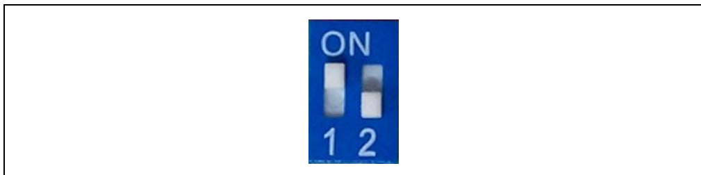
FIGURE 3-31: SWITCH SW9 IN FLASH TEST MODE
