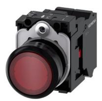
Illuminated pushbutton, 22 mm, round, plastic, red, pushbutton, flat, momentary contact type, with holder, 1NC, LED module with integrated LED 110 V AC, spring-type terminal, with laser labeling, upper case and lower case, Always upper case at the beginning of the word
