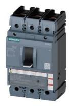
circuit breaker 3VA5 UL frame 250 breaking capacity class M 35kA @ 480 V 3-pole, line protection TM210, FTFM, In=80A overload protection Ir=80A fixed short-circuit protection Ii=10 x In UL489 SB (naval), 50 deg. cel. nut keeper kit on both sides
