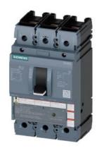
circuit breaker 3VA5 UL frame 250 breaking capacity class C 100kA @ 480 V 3-pole, line protection TM210, FTFM, In=100A overload protection Ir=100A fixed short-circuit protection Ii=10 x In nut keeper kit on both sides
