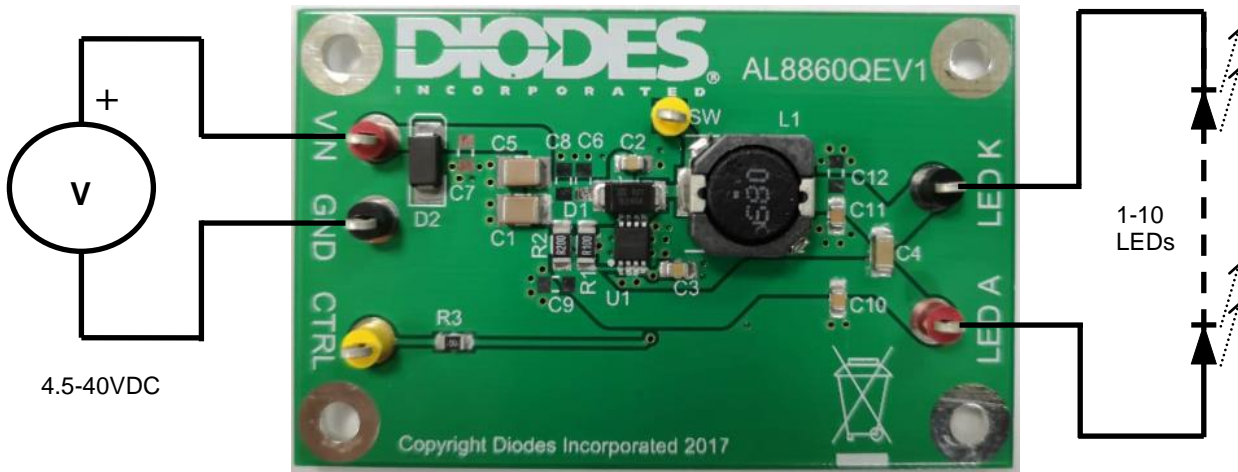
Figure 1: AL8860QEV1 evaluation board and connection diagram
