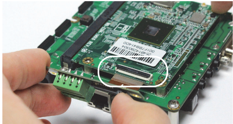
Figure 31: Connecting adapter board and embedded board
