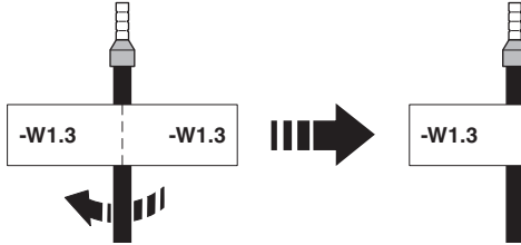
Figure 4-7 Example of a cable flag
