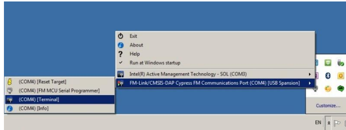
Figure 2-7. FM-Link/CMSIS-DAP Cypress FM Communications Port
