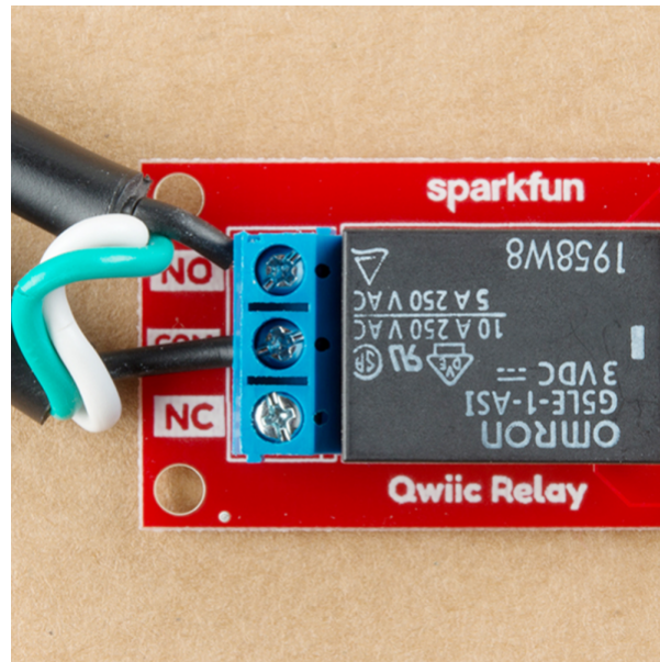
Relay Example Connection
