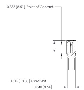
746 Series Ultra-Mate Card Edge Connector - Press Fit Part Number: 746-056-545-201
