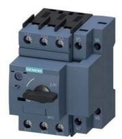
Circuit breaker size S00 for motor protection, CLASS 10 with overload relay function A-release 0.45...0.63 A N-release 8.2 A screw terminal Standard switching capacity
