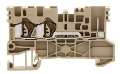
Feed-through terminal, Tension-spring connection, Mounting type: Mounting rail TS 35/7.5, Rated cross-section: 2.5 mm², Width: 5.1 mm, Colour: Beige
