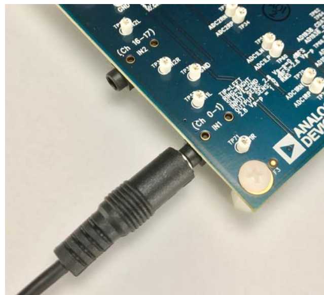
Figure 11. Analog Stereo Input Source Connection
