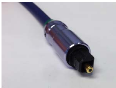
Figure 61. TOSLINK Connector and Optical Fiber Cable for S/PDIF Input and Output
