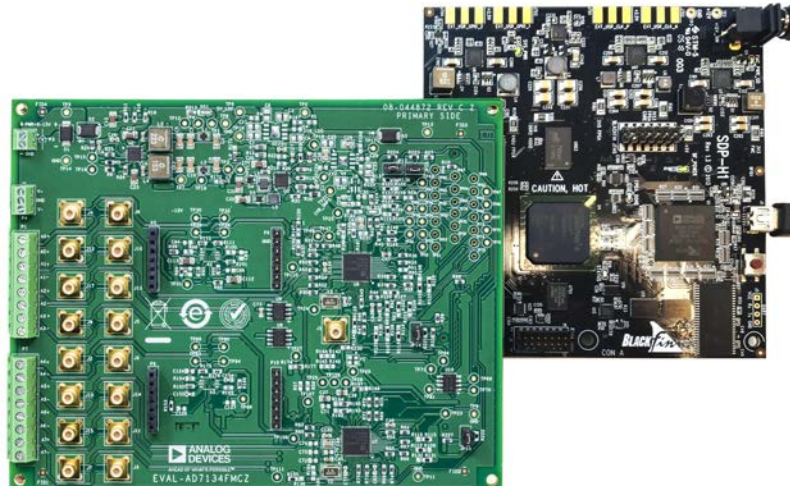
Figure 2. EVAL-AD7134FMCZ and SDP-H1 Board Connection
