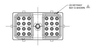
24 POS, PLUG, SOCKET, ARC SERIES, KEYED, RD SEAL, BLACK
