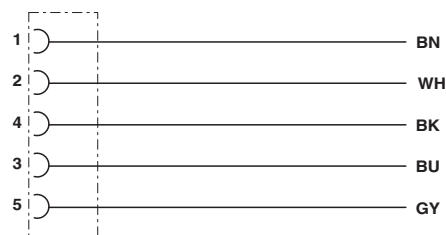
Contact assignment of the M12 socket
