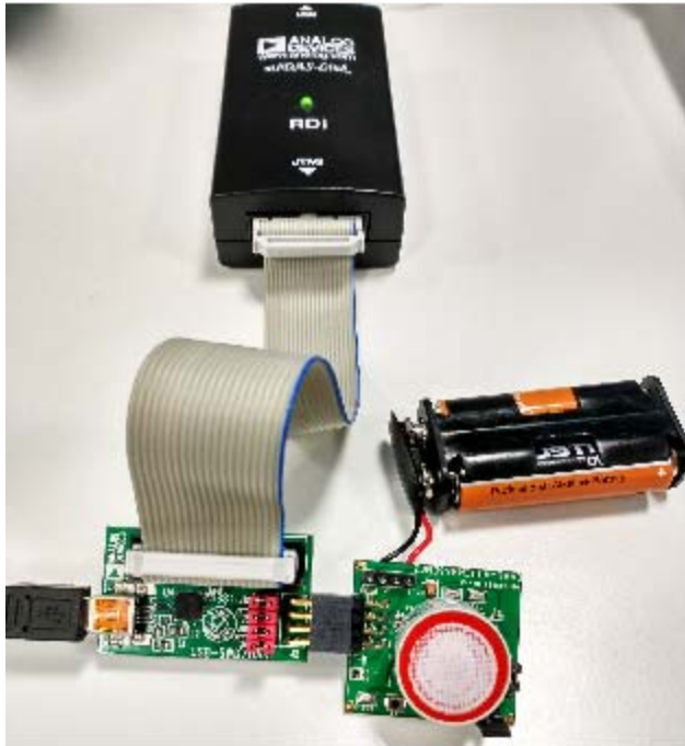
Figure 9. Connecting Programming/Debugging POD to the EVAL-ADuCM355EMCZ
