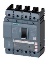
circuit breaker 3VA5 UL frame 250 breaking capacity class C 100kA @ 480V 4-pole, line protection TM230, FTAM, In=80A overload protection Ir=80A fixed short-circuit protection Ii=5...10 x In N conductor unprotected without connection
