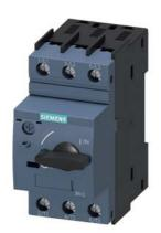
Special type Circuit breaker size S00 for motor protection, CLASS 10 A-release 10...16 A N-release 208 A screw terminal Standard switching capacity Ambient temperature -50  $^{\circ}$ C 500 switching cycles
