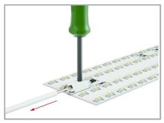
Inserting/removing solid conductors by lightly pressing on a push-button.
