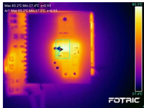
a) NV6125 (90 VAC, 100% Load)
