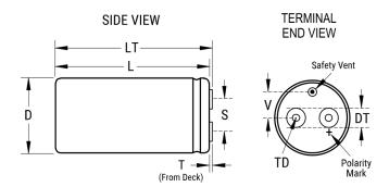
General Information Series ALS30 Dielectric Aluminum Electrolytic Description Screw Terminal, Aluminum Electrolytic RoHS AEC-Q200 No Component 115 g Weight Dimensions D And L Include Sleeving. MS (MxH) = Notes M8x12. Mounting Clamp (Sold Separately): V3/H2/2736 Shelf Life 156 Weeks
