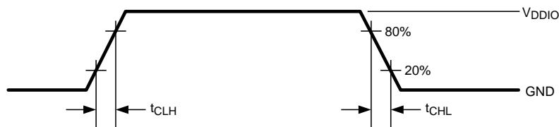
Figure 10. Deserializer LVCMOS Transition Times
