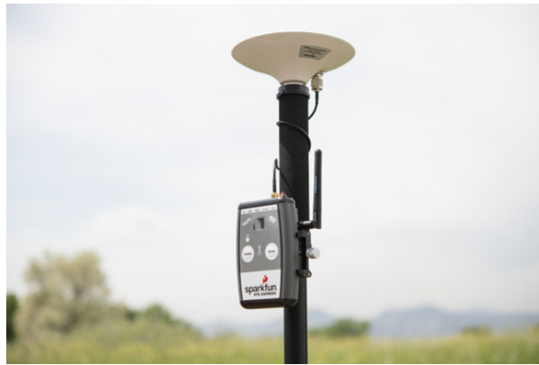
2nd most common setup with a 915MHz Radio providing RTCM
