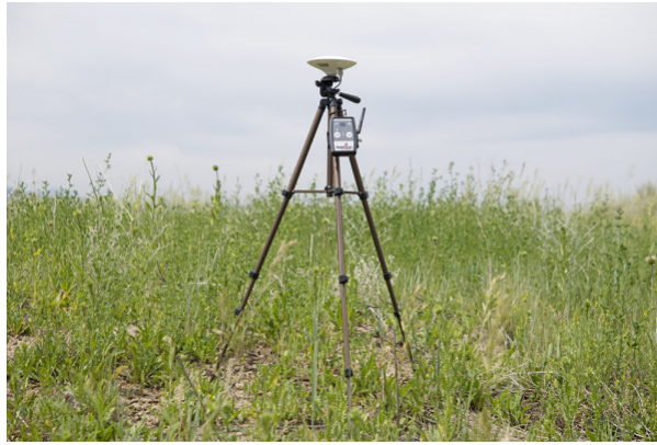
Temporary RTK Express Base setup
