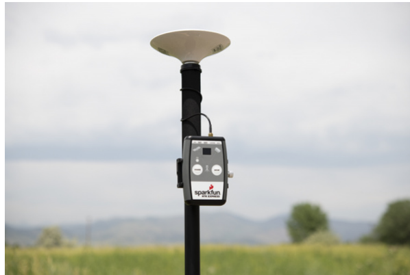
Basic RTK Express Rover setup with RTCM over Bluetooth
