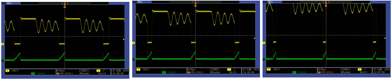
Figure 2-4. Drain Voltage and Drain current waveform (VO=24V,IO=1.0A, PO=24W)
