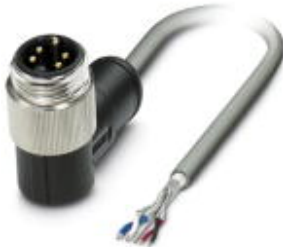
Bus system cable, DeviceNet, 5-position, PUR halogen-free, Gray RAL 7001, Plug angled 7/8"-16UNF, on Free cable end, Cable length: 5 m
