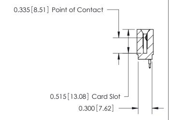
ACAD REFERENCE NO. 745 Series Ultra-Mate Card Edge Connector - Press Fit DRAWN: J.LEE Part Number: 745-036-525-101 CHECKED: **EDAC INC** SCALE: THESE DRAWINGS AND SPECIFICATIONS ARE THE PROPERTY OF EDAC INC.,AND TORONTO, ONTARIO SHALL NOT BE REPRODUCED, OR COPIED DRAWING NUMBER CANADA OR USED AS THE BASIS FOR THE 745-ENG MASTER MANUFACTURE OR SALE OF APPARATUS YOUR CONNECTION TO QUALITY & SERVICE WITHOUT WRITTEN PERMISSION.
