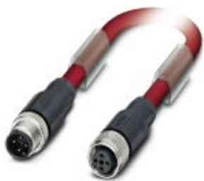
Bus system cable, CC link (10 Mbps), 4-position, PVC, red, shielded, Plug straight M12, A-coded, on Socket straight M12, A-coded, cable length: 5 m
