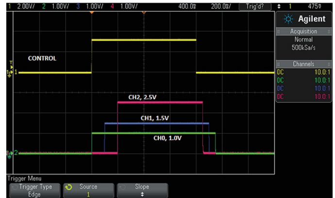
Figure 6. Sequencing Output Channels On/Off
