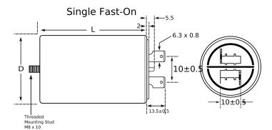
Series C27 Dielectric Film/Foil Polypropylene Style Plastic Case and Cover, Ultra Sonically Welded Description Ultra Sonically Welded Seal, Safety Class PO, Features UL 94 V0 Disk **RoHS** Yes Lead Fast On (1+1) UL, VDE, UL (Construction Only), UL\_94 VO Qualifications Disk AEC-Q200 No Component 112 g Weight
