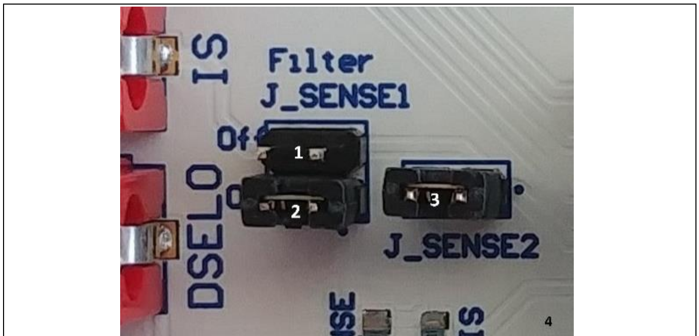
Figure 3 Jumper setup of J_SENSE
