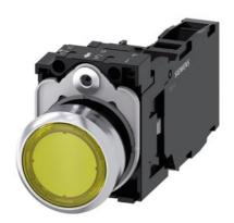
Illuminated pushbutton, 22 mm, round, metal, shiny, yellow, pushbutton, flat, momentary contact type, with holder, 1 NO+1 NC, LED module with integrated LED 230 V AC, screw terminal, Z=20-unit packaging
