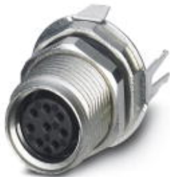
Sensor/actuator flush-type plug-in connector, socket, 8-pos. M8, rear/screw mounting with M10 fastening thread, with straight solder connection
