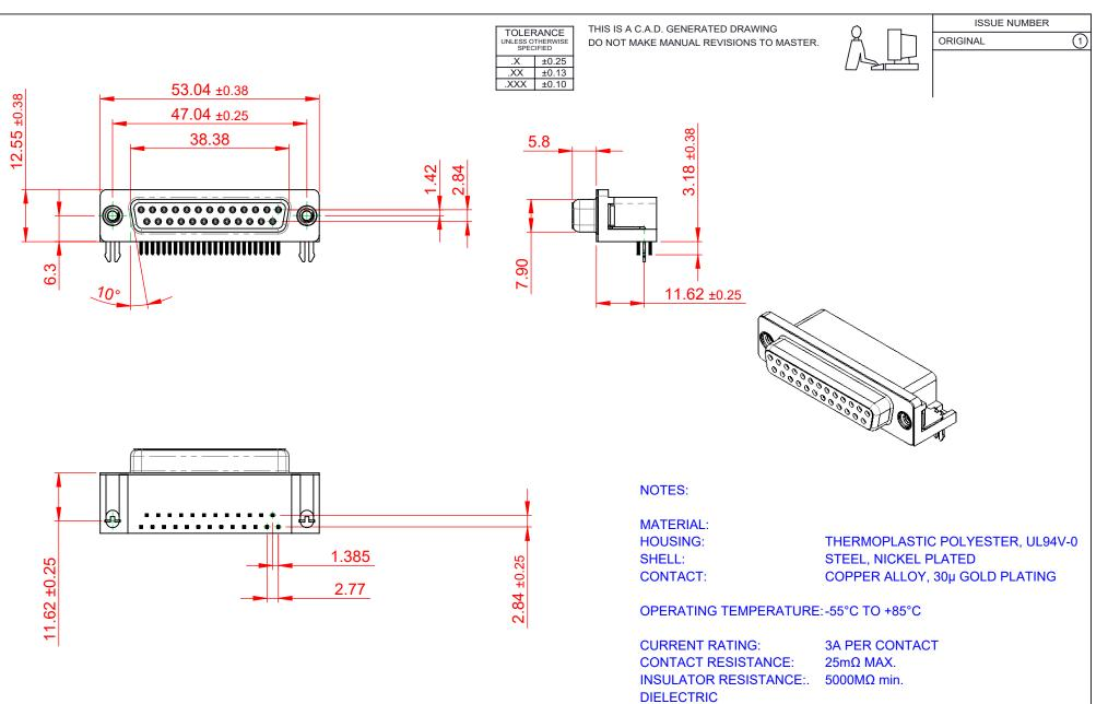
WITHSTANDING VOLTAGE: 1000V AC rms
